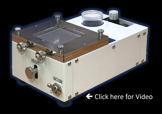
The tool is designed to address reduced time and cost saving, stabilizing the manual alignment of X, Y, Z, and  $\theta$ , and reducing costs by eliminating the need of designing a nest for each and every single component.
